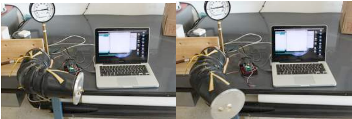
Figure 14. Robotic Arm Cycling of Arm #15. Flexion (R) and Extension (L)
