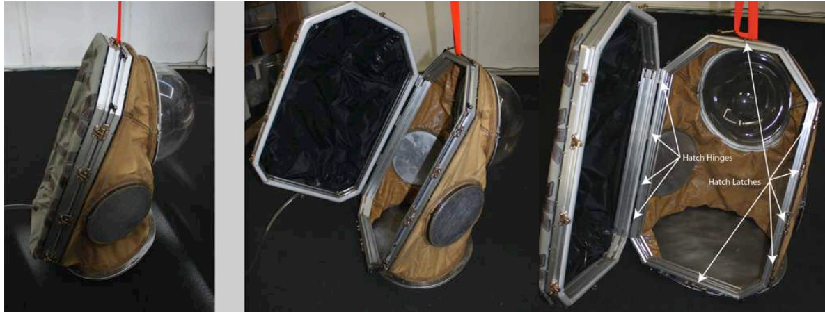
Figure 6. SRUT Hatch closed (left) and open (middle), showing hinges and latches (right)
