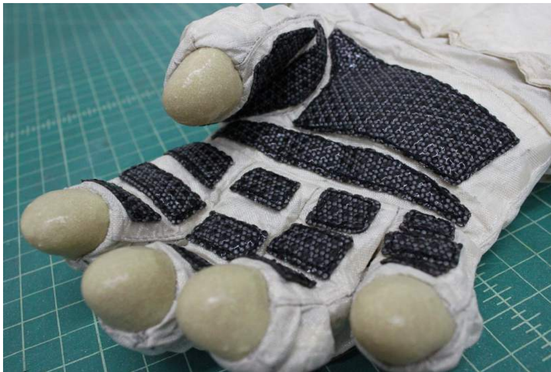
Figure 26. FFD’s EVA Outer Garment Glove Palm with Superfabric
