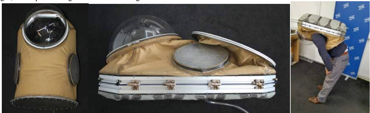
Figure 7. SRUT prototype evaluation - pressure, stowage, donning/doffing and range of motion
