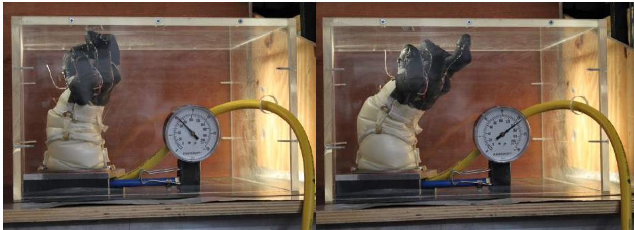
Figure 18. FFD’s Pressure Garment Glove at +10.6 psid (left) and +21.2 psid (right).
