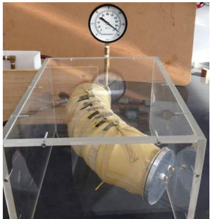
Figure 9. FFD's Elbow #16, inflated to +29 psid
