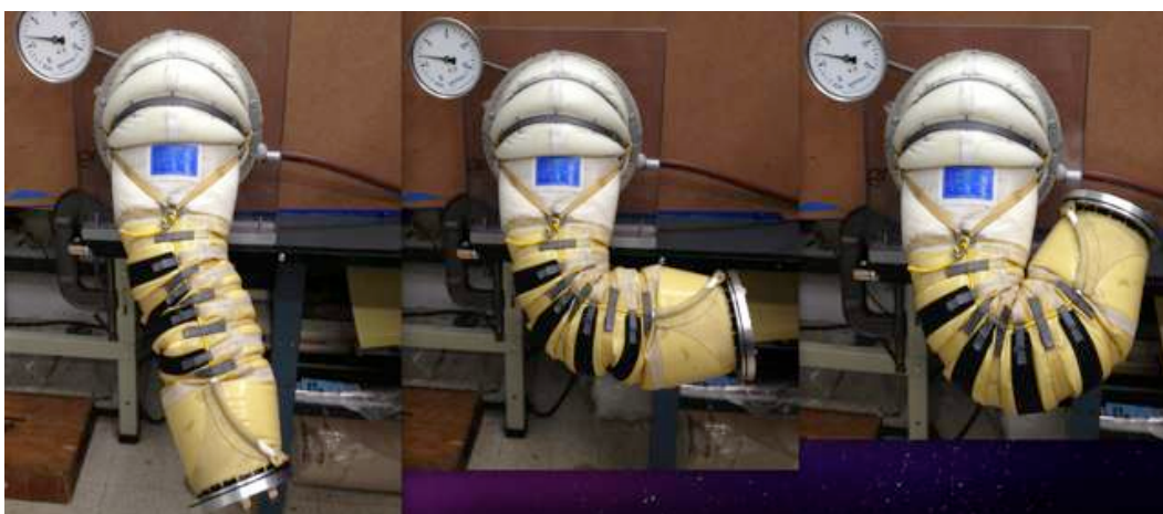
Figure 15. FFD's elbow and shoulder assembly at +4.3 psid
