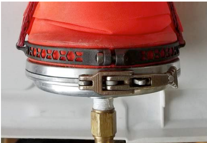
Figure 27. FFD’s Glove quick disconnect
