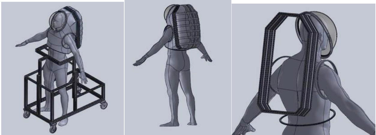
Figure 4. Isometric view of ESSE, showing a cart, backpack, and interface orientation
