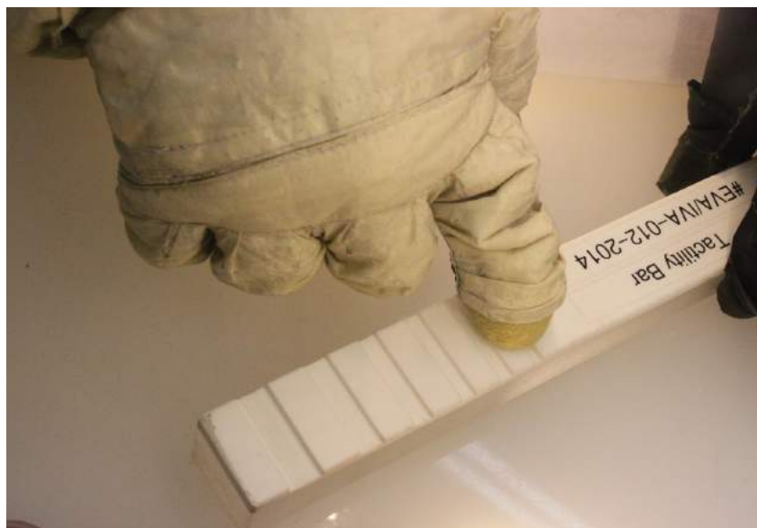
Figure 25. Fingertip tactility testing to 0.1875" with TMG at 8 psid
