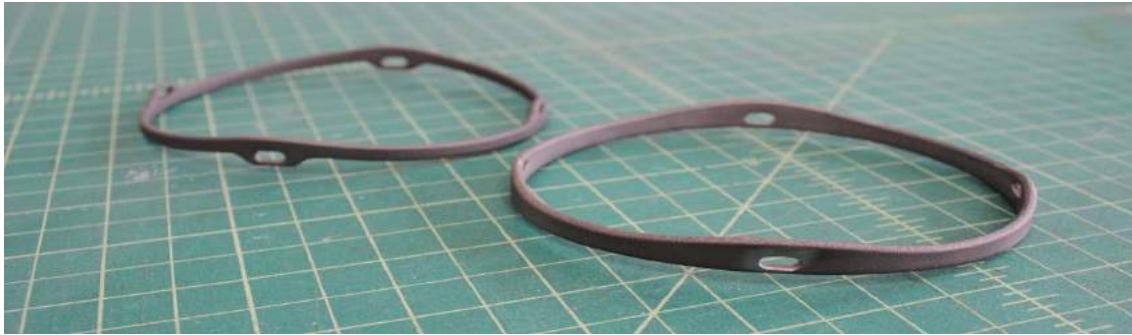
Figure 20. Gimbal Ring Optimization. Original Ring (Left) and Reinforced Ring (Right)
